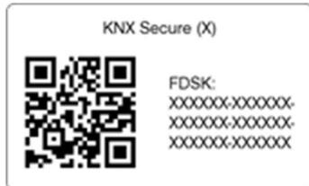
Neither the FDSK nor the tool key are transmitted in plain text. Once the transfer is complete, the device will only accept the **tool key** for project configuration. The FDSK is only required again if the device is reset to factory settings.
