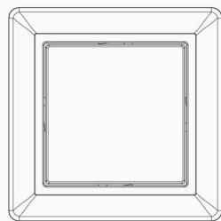
Integrated in switch design 55 x 55 mm
